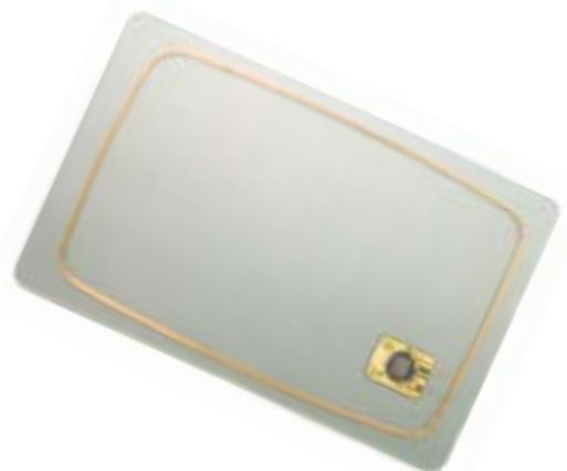
The MIFARE Cards can handle multiple applications. Every sector can carry information for a different application. On the 1K MIFARE cards each sector is divided into 4 blocks of information; each block can contain 16 bytes of data; block 3 of each sector is used for key storage and access conditions for that particular sector.
