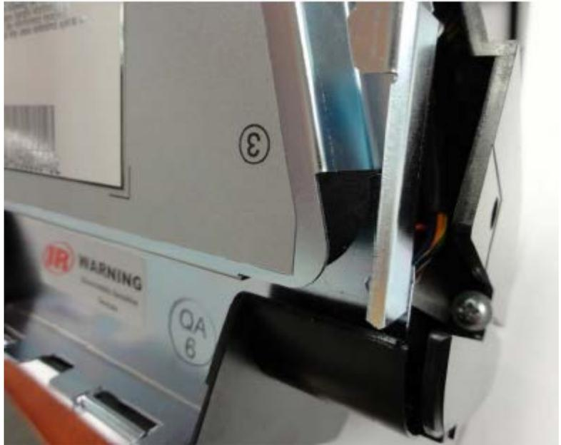
Pull the backup battery cable through the back plate as shown above.
