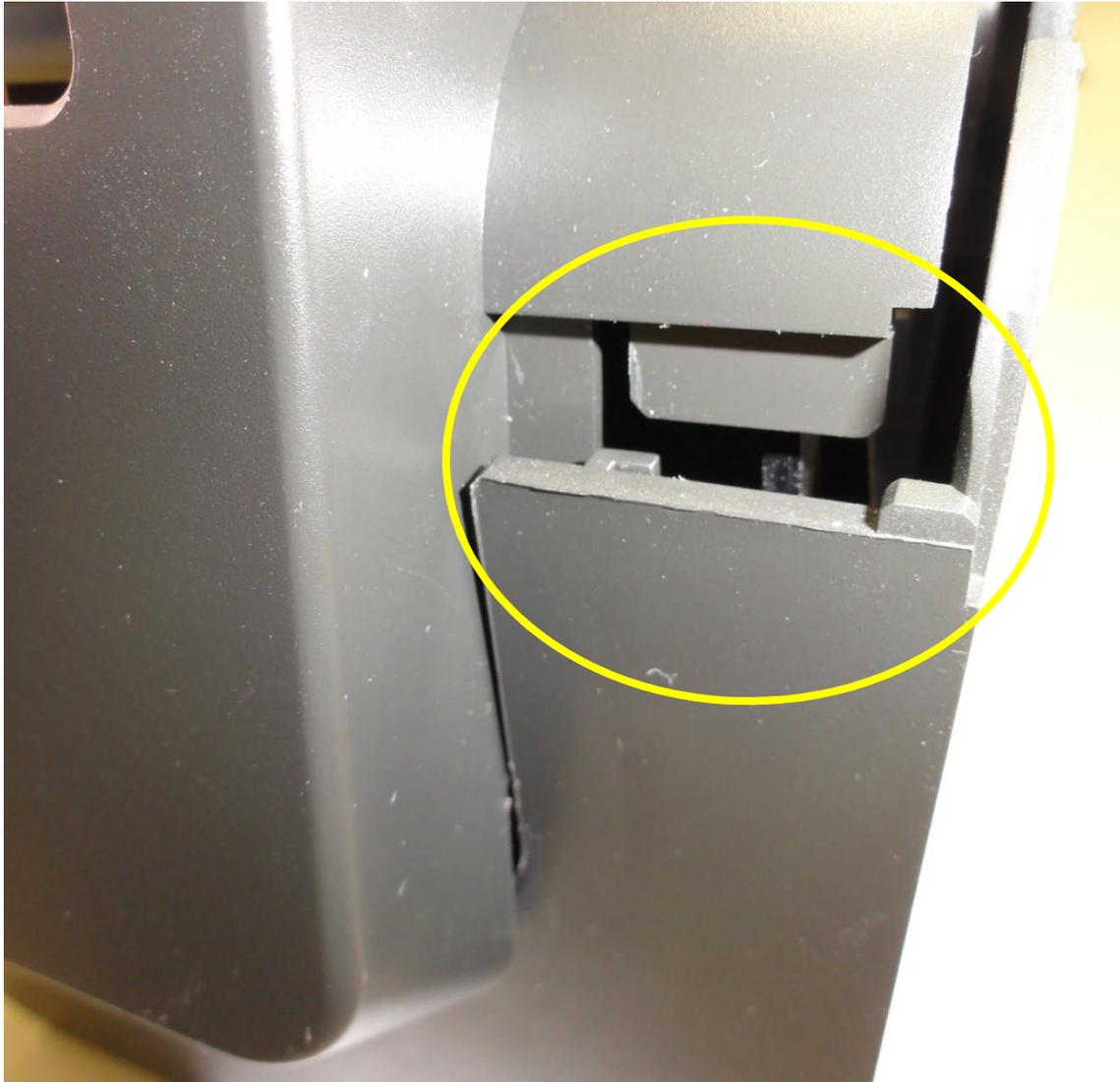
Slide the battery compartment back into the bottom of the unit slide the battery compartment so that it mates up. Press the battery compartment in so that it is flush in place.
