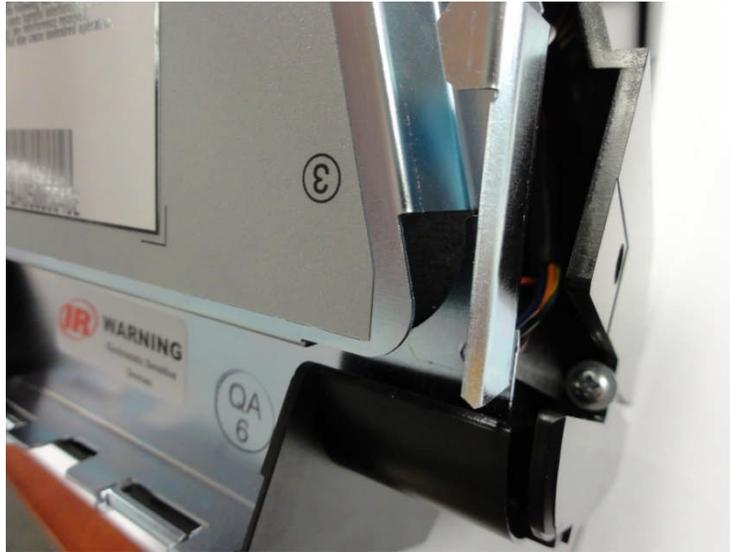
Start with setting the back plate into the battery compartment and start rotating the back plate towards the top. Make sure that the BB-300 cable is not getting pinched in the lower right hand cable. Stop when you get to the camera cable.
