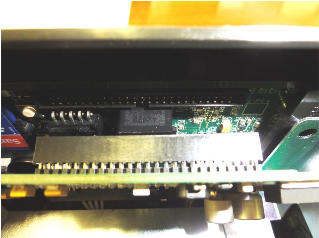
Making sure your ground strap is on. Align the 2 x 25 pin connector and header and gently mate the two boards.
