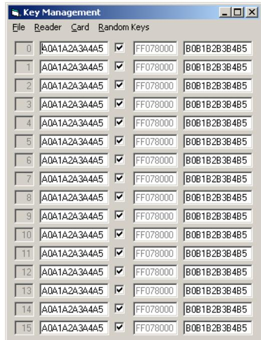
The relevant keys should be typed in HEX format (0 – 9, A – F) on position 2 and 3. The first key is the “A” key for reading information the second the “B” key for writing information to the card. The field in the middle is the access conditions for the sector. For our purpose: Key Upload they are not relevant.
